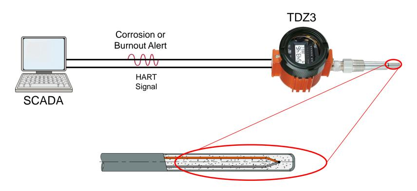
TC junctions start to break down before burnout - an increase in the junction resistance can be an early indication of TC degradation or pending failure
